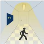
When motion detected, insufficient daylight, Light ON.
