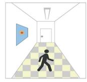
When motion detected, but sufficientdaylight, Light remains OFF.
